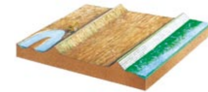
If no high ground is present inland, a new flood bank is built behind the existing one. The land is managed to ensure the right habitat is created.
